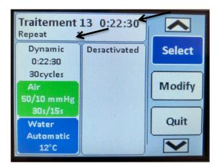
Click on the time of the working cycle. Set the cycle time, for example for a 30-minute period. Click on "Validate".
